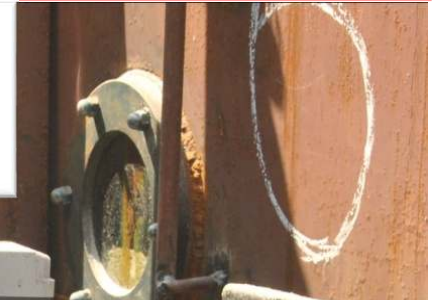
Auto Retracting Self Cleaning Brix Sensor installed on Continuous Vacuum Pan & Sugar Melter in Picture below
