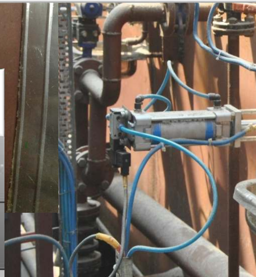
Auto Retracting Self Cleaning Brix Sensor installed on Continuous Vacuum Pan & Sugar Melter in Picture below
