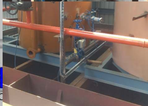
Auto Retracting Self Cleaning Brix Sensor installed on Batch Type Vacuum Pan
