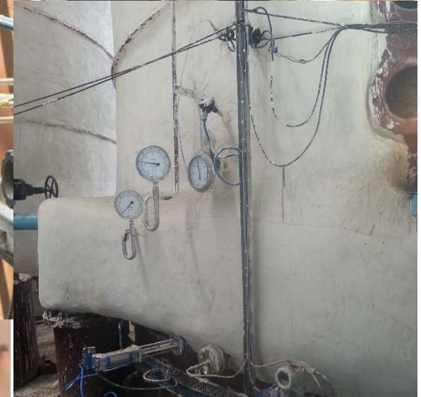
Auto Retracting Self Cleaning Brix Sensor installed on Batch Type Vacuum Pan
